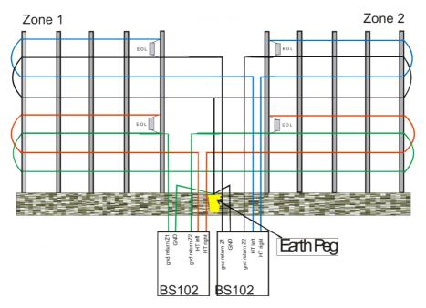
Several earth points can be connected to the earth wire along the fence without interfering with the ground loop protection.
