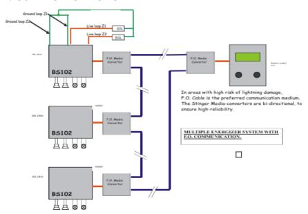
Communication to master, slave control units, or computer can be only done via copper cable if there is no danger of lightning damage.
